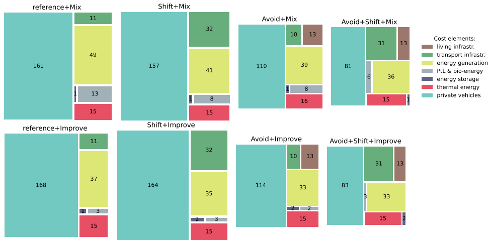
Figure 4.7: Scenario cost by component. Private vehicle stocks make up the largest share and increase in Improve scenarios. Shift and Avoid scenarios add infrastructure cost for public transport and living (multiplex buildings, provisioning), making cost without private vehicles exceed the reference. Energy system cost decrease stronger on the transport supply axis (vertically) than on the transport demand axis (horizontally) due to less Power-to-Liquid (PtL) facilities and corresponding renewable energy generation.
