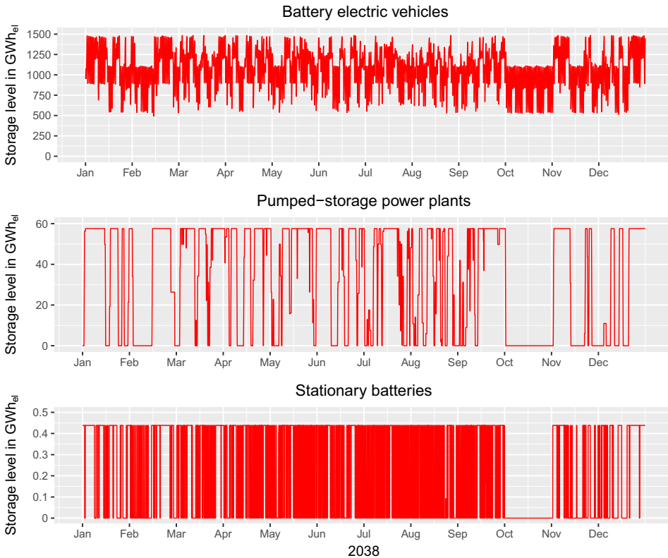
Figure 6.38: Charge levels of power storages in 2038. The wind speed and the solar radiation in October are set to zero for Germany and its neighbouring countries.
