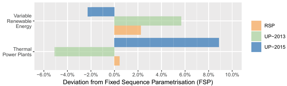
Figure 6.34: Variation of installed capacity of power generators for differing parametrisation of weather data related to the Fixed Sequence Parametrisation. UP-2013: Uniform Parametrisation 2013, UP-2015: Uniform Parametrisation 2015, RSP: Random Sequence Parametrisation.
