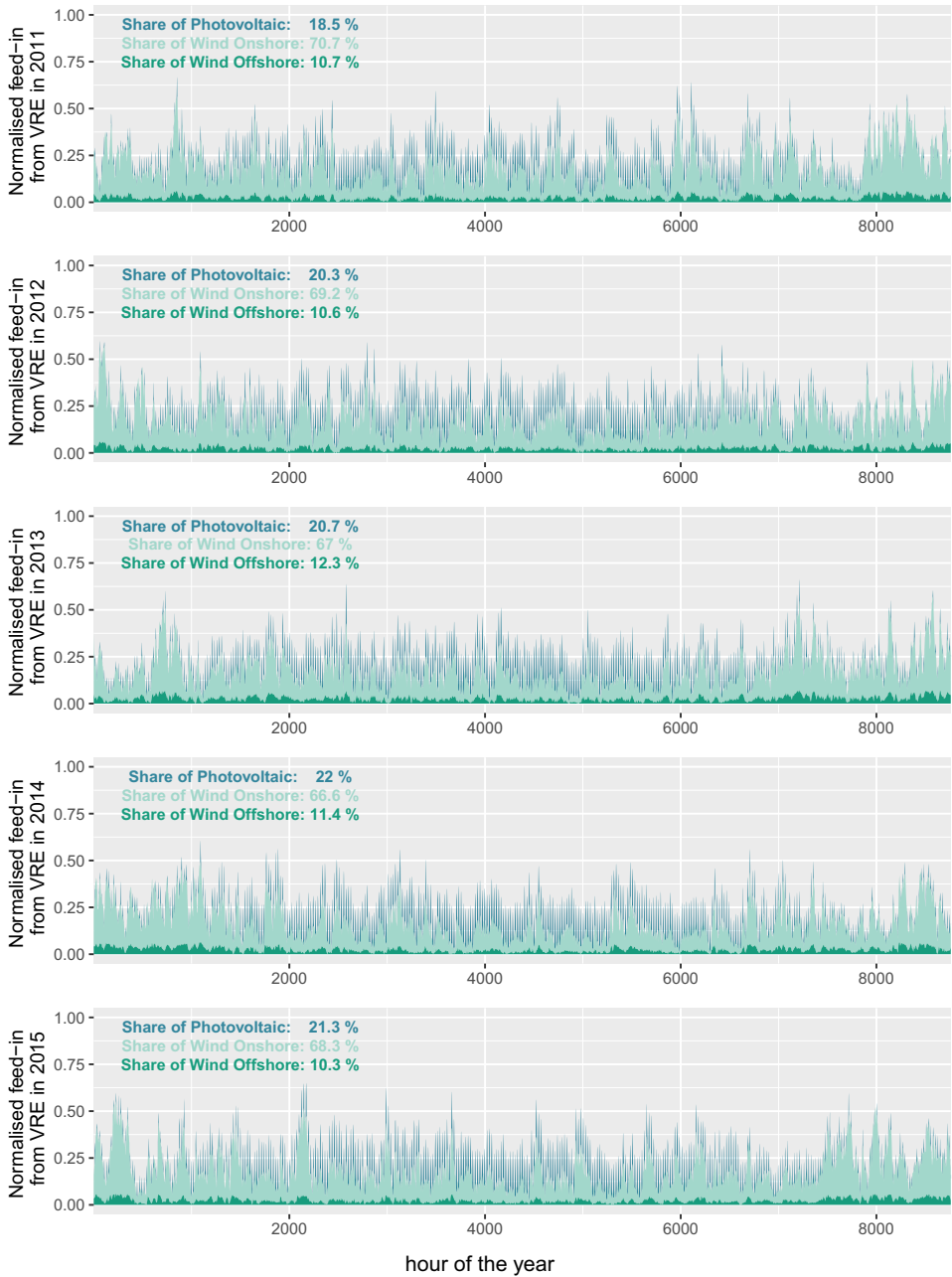
Figure 4.13: Normalised power supply profiles for photovoltaic systems, onshore and offshore wind power stations for Germany's neighbouring countries and five weather data sets for the years 2011 to 2015.
